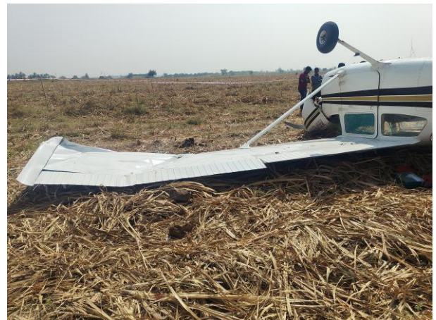
Damaged RH wing
